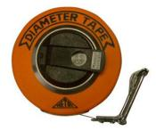
(Figure 2. diameter tape)
